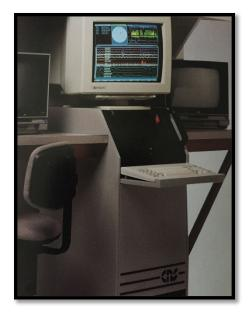
The Computer Aided Sleep System (CASS) was introduced to the sleep lab market in 1985. It replaced the polysomnography (and paper), but digitizing the data and performing automated analysis of the data with editing capabilities. CASS measured all of the parameters typically measured in a sleep lab.
