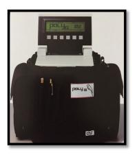
The  $Poly_G$  System was introduced to the sleep lab market in 1989. It was a novel portable device that could be sent home with the patient to screen for sleep apnea.  $Poly_G$  measured respiratory flow and effort as well as blood oxygen levels.
